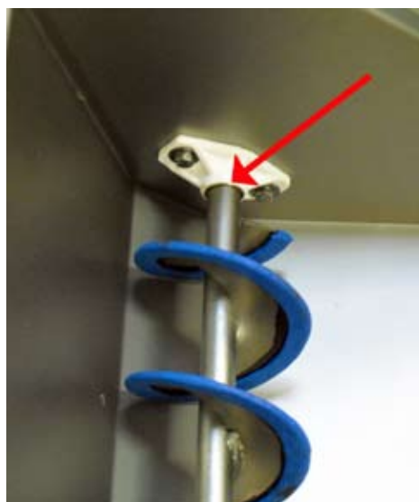
Fig. 8. Lubricate the bushing in hopper annually.
