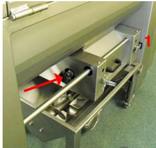
Fig. 3. Turn black knob to disconnect rollers.
