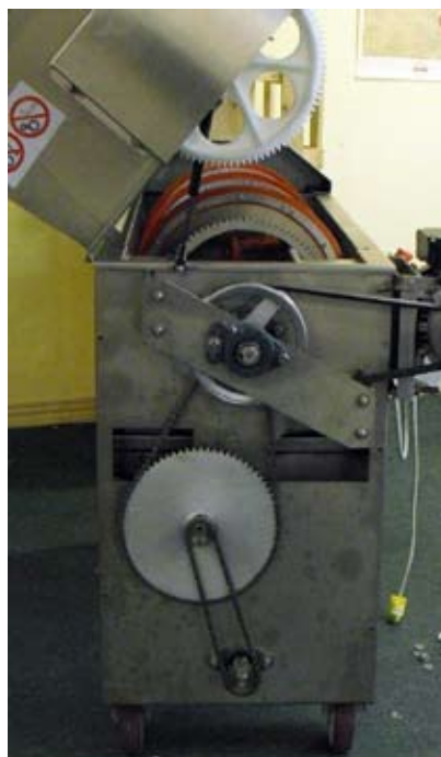
Fig. 9. Remove end cover annually and lubricate chains and gears. To not grease the V-belts. Do not wash down these components.
