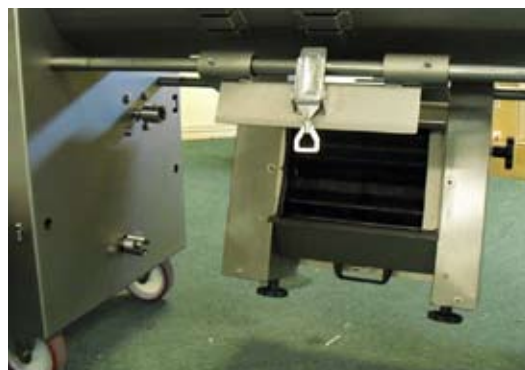
Fig. 5 Rollers drop down for easy cleaning.
