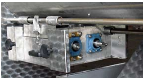
Fig. 4. Roller bearings exposed when side panels are removed. Remove side panels to lubricate. Do NOT pressure wash bearings.
