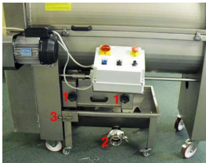
Fig. 2. "1" are roller adjustment knobs. "2" is outlet (3" TC) for must pump. There is an identical outlet on other side. Choose whichever side is most convenient. "3" is a latch. The rollers and outlet basin are latched in position.
